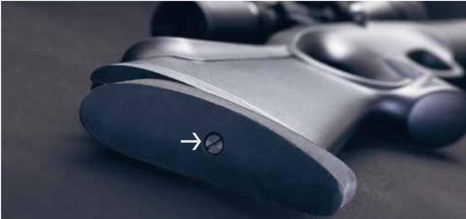
**Model 16051:** Loosen the screw in the middle (seen on the picture) to be able to move the recoil pad. Tighten screw when recoil pad is in desired position.
