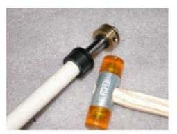
There will probably be marks on the barrel from the three screws holding it, grind these down.
