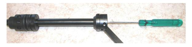
**5.** Lock the inner rod 19089 with screw 2534, see picture below.
