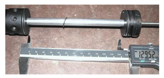
**3.** The tube 19090 Needs to be tightened to Tube end 19049 and in the other end you should adjust the distance with big piston 19046 to 125,1mm - 125,3mm, see picture below.
