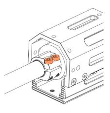
5. Unscrew plenum tube (D-A11) which is threaded to main block (D-B9).You might need to clamp the tube carefully in a vice do be able to loosen it.This will make the barrel visible and make it easier to continue your work.
