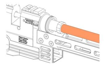
6. Loosen the two locking screws for the barrel (D-B11). These can be somewhat tricky as they are loctited/glued in place. Use <u>quality tools</u> and apply heat (gently) if necessary. Gently remove barrel from its' slot.
