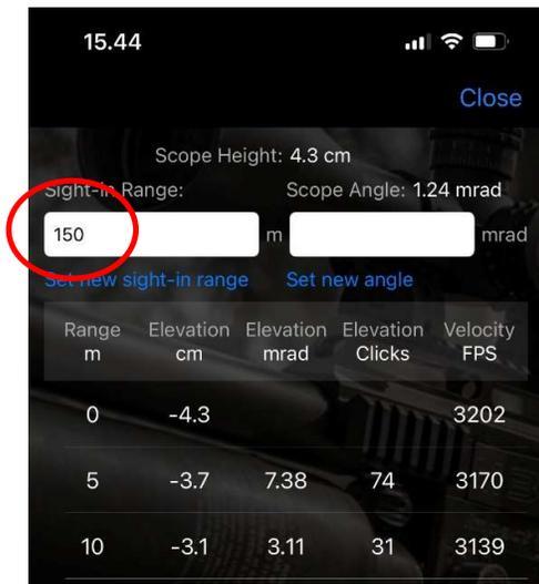
On the top right, you will see the **calculated scope angle** for your current elevation turret position, which in this example is 1.24mrad. You can round this value to 1.2mrad if you want, since it is not possible to adjust the elevation turret in increments of 1/10th of a click. Once you have the calculated scope angle, set it to the scope angle field and use it instead of the sight-in range.
