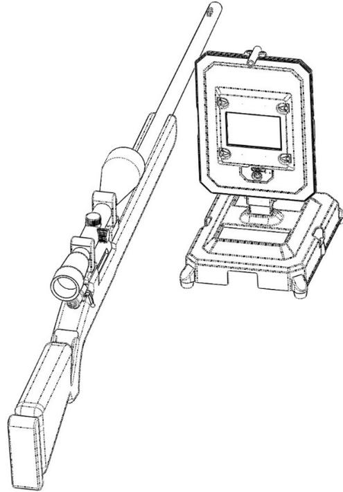
If the chronograph needs to be positioned away from the barrel, make sure to set the correct Barrel Offset in the configuration menu. The default setting for Barrel Offset is 0"-8". This ensures that the chronograph accurately measures the bullet's velocity.
