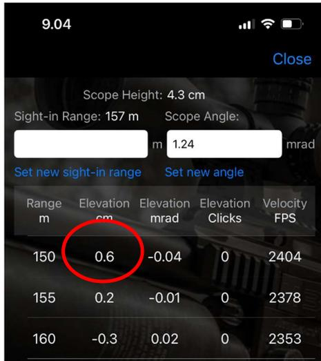
If you need to change your scope angle for any reason, it is easy to do. For example, if you want to set the scope angle of this example to 1.0mrad, which may be easier to remember, you can simply adjust the elevation turret down by two clicks and then reset the turret zero to the new position. In this example, a Mil Dot scope is being used, and one click of the scope equals 0.1mrad. In the case of a MOA scope, one click would equal 0.25 MOA.
