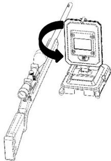
If the chronograph is positioned on the right side of the gun, it is better to **rotate it slightly counterclockwise** to ensure that the transmitted radar signal crosses the bullet's trajectory. Rotating the chronograph clockwise may result in the bullet never entering the strongest area of the radar signal.
