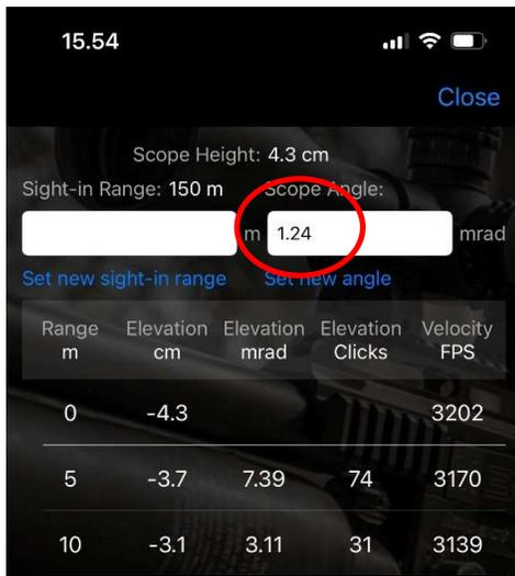
The advantage of using the scope angle instead of the sight-in range is that you can shoot any bullet and get a correct ballistic solution regardless of the actual sight-in range for the bullet. **The elevation clicks reported in the app are based on the elevation turret zero position.** This means that by using the scope angle instead of the sight-in range, you can shoot any bullet and get a correct solution without needing to adjust the sight-in range for each bullet.
