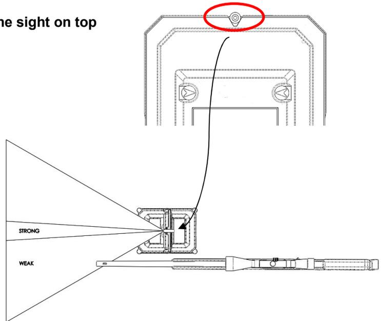
If the chronograph is not positioned with a clear line of sight to the muzzle, it will trigger slightly after the bullet exited the muzzle and will not be able to accurately measure the velocity at the muzzle.
