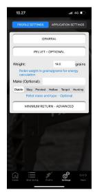
3. The "Minimum Return" setting in the "Advanced" section of the settings is rarely needed. In some cases, the sensitivity of the chronograph may need to be adjusted. If a shot is not being registered, you can try lowering the minimum return value to make the chronograph more sensitive. If the chronograph is reading random values, you can try increasing the minimum return value.
