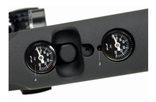
**3. Externally Adjustable Regulator** – In the stock beside the front pressure gauge there is a machined slot where the regulator adjustment screw is located. Tool required for adjustment: 2,5 mm Hex key.
