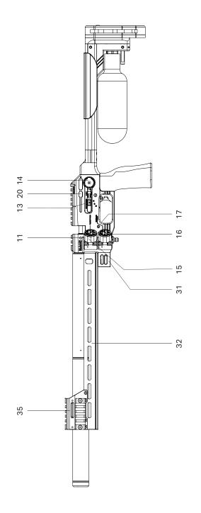
11 Barrel Fastener (do not tamper with) 13 Micro Power Adjuster 14 Macro Power Ajuster 15 Regulator Pressure
