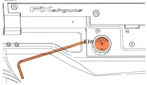
The regulator reduces the pressure and sets the output/working pressure for the rifle.
